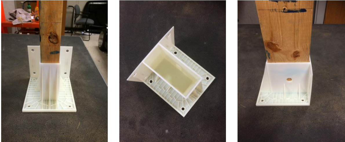
Figure 19: Different views of the 3D printed 2x4 adaptor
